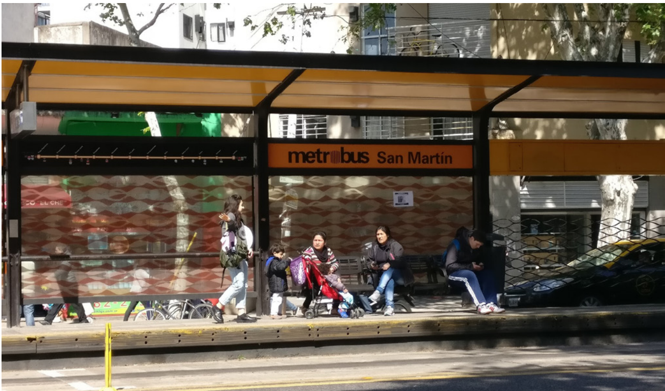
Figure 46. Waiting at San Martín Metrobus station, a well-designed bus stop (similar to a station) with clear sight lines, seating, good passenger and real time information. Photo credit: Sebastián Anapolsky.
